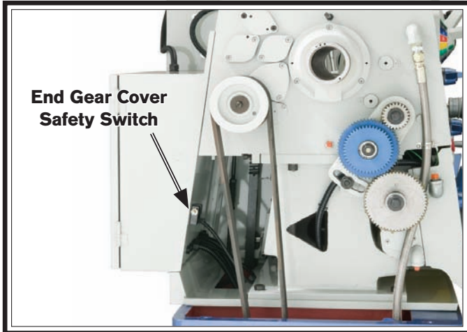
Figure 143. End Gear Cover Safety switch location.
